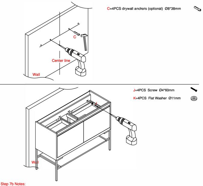
Secure the cabinet to the wall using hardware J (screws) and Flat Washer K for wall studs.
